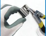
Place the tip of the C Clamp Pliers into the installation hole in the Constrictor's face and open. **NEVER open the Constrictor wider** than the Nexthermal Custom C Clamp allows.
